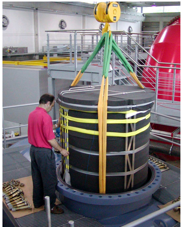
FIG. 4: The High-Pressure Convection Facility, weighing approximately 2000 kg, is being inserted into the turret of the Uboot.
