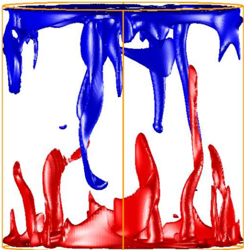
FIG. 3: Visualization for Ra = 10^8 of two temperature isosurfaces in a cylindrical sample with \Gamma = 1 for Pr = 6.4 and at a modest rotation rate. From [30].
